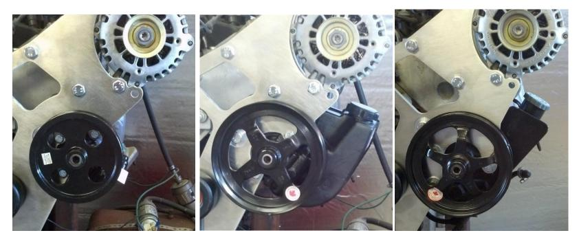
Left: Type II pump with 5.5" pulley and 90 degree hose barb for remote reservoir. Can work with any balancer. Available from Kwik Performance, part number 10206-03.
